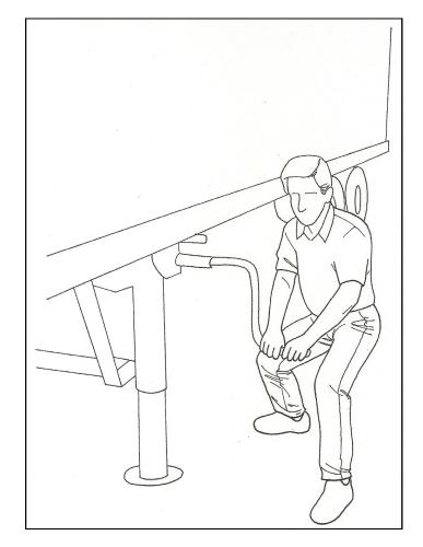
Using the crank to roll dolly legs up and down is another perfect example of POWERLIFT® technique. Here, instead of cranking with your back, you can easily use your legs. Simply stand at a 45° angle to the crank with a wide stance. Use your legs for the power to turn the crank, rather than your back. Remember that this technique works great whether using one hand or two hands on the crank. Use wide stance whichever way you face the crank so that your back stays out of this lift.
