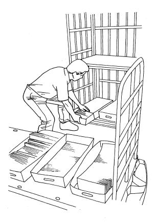
Desleeving trays is a job that should only be done in wide stance. The amount of bend/twisting associated with this task can be very significant if you are using your back for the job. Remember that with wide stance, knees bent, the bend/twist takes place in your hips and pelvis where it belongs, rather than in your back.
