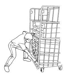
The first task of desleeving involves cutting the plastic straps. For this, stand at a 45° angle to the front of the stack of trays in wide stance, with your knees bent. Note as in the illustration, you can use your free hand to stabilize yourself while bending down to cut the straps. Notice also, that in this position your range of motion is greatly improved and you can reach to almost any area without moving your feet.
