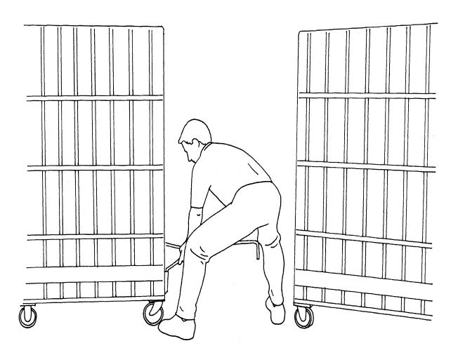
To place the hook, always use two hands and step in front of the container with a 45° wide bent knee PowerLift® stance.
