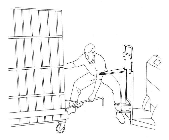
The container may have to be pulled into position. To pull the container into position, never leave your feet close together; this will force you into using your back to maneuver the container into position. Maintain a wide 45° bent knee PowerLift® stance and pull with your legs.
