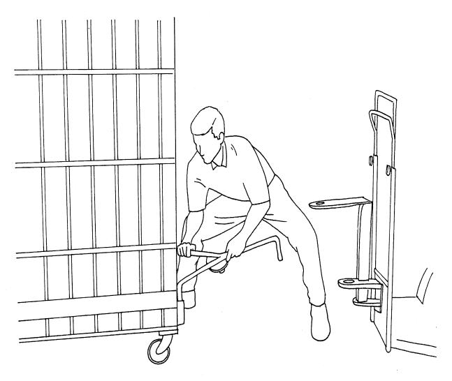
When hooking together wheeled containers such as APCs, GPMCs, OTRs, and Hampers always use a wide stance. You will find there is plenty of room between containers to allow one of your legs to step into a wide 45° bent knee PowerLift® stance.
