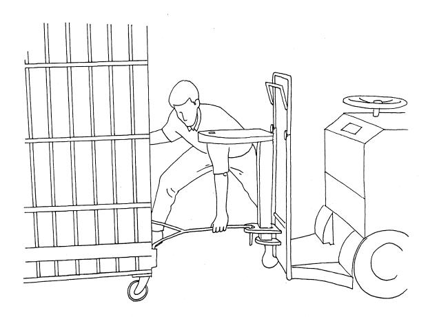
Use one hand on the container and one hand on the hook to pull the wheeled container into position and hook them together.
