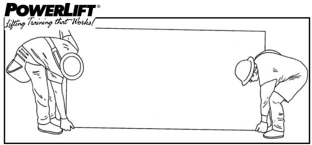
In observing these workers, you can truly see that they both are using a <u>narrow</u> stance and a back lift to transfer this sheet of Gypsum.
