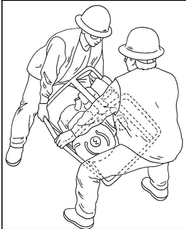
These two workers are lifting the pump the hard way. They are doing a half-back/half-leg lift. Your legs are not nearly as strong in this position and it pulls your back into the lift.
