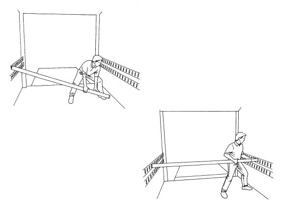
For load bars, never lift with your back. Rather, use a wide stance POWERLIFT® approach for lifting and positioning.
