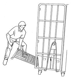
When opening the bottom gate on the GPMC it is really easy to use your back simply because you have to bend all the way to the floor to handle the gate. It can be just as easy to use your legs if you remember to stand at a wide stance with your knees bent and allow the corner of the gate to pass between your knees as it folds down.
