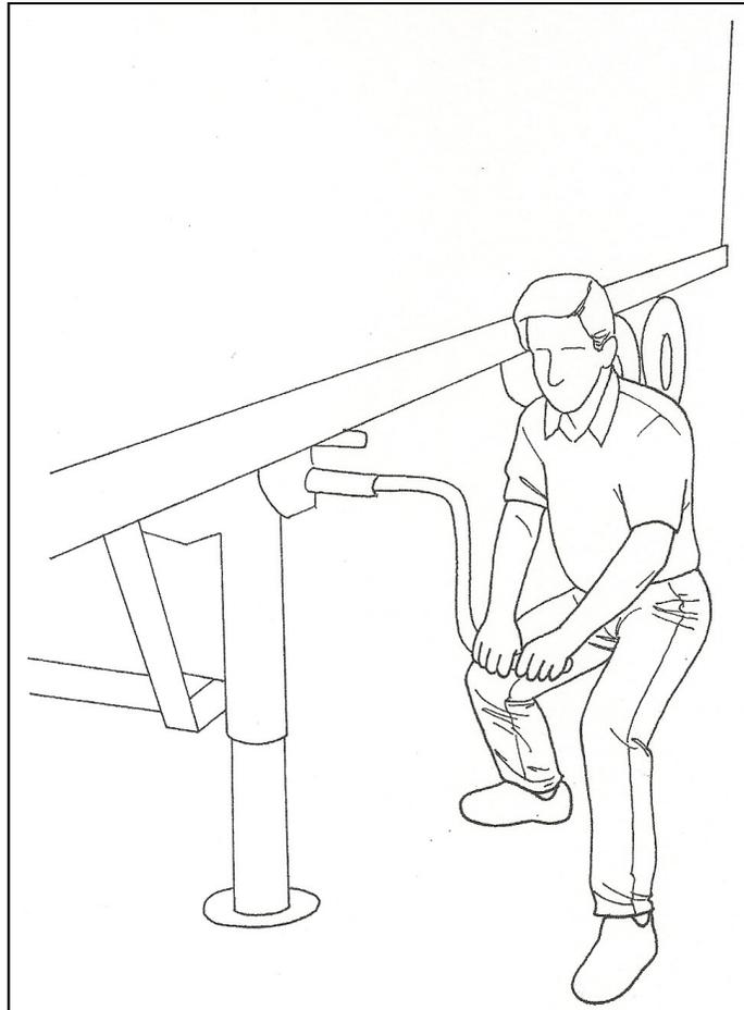
Using the crank to roll dolly legs up and down is another perfect example of POWERLIFT® technique. Here, instead of cranking with your back, you can easily use your legs. Simply stand at a 45° angle to the crank with a wide stance. Use your legs for the power to turn the crank, rather than your back. Remember that this technique works great whether using one hand or two hands on the crank. Use wide stance whichever way you face the crank so that your back stays out of this lift.
