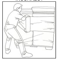
Note in this illustration that the wrap is being applied from right to left. Note also that the worker's left arm is on the bottom of the shrink wrap roll with his right hand at the top. This combination of elements (right to left motion, left hand bottom and right hand top) results in a bend/twist to the back as this job is being performed.
