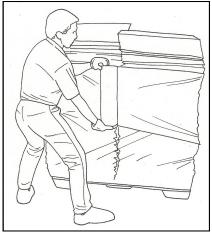
Never, ever, bend/twist your back, even with this simple job. Note in this illustration, as the wrapping proceeds from right to left, the worker's right hand is at the bottom of the roll with the left hand at the top. This allows the back to remain upright and not in a twisted position. Although this may seem like a trivial point, it is the bend/twist position that can easily kink a back. Always use wide stance POWERLIFT® to avoid bend/twist.
