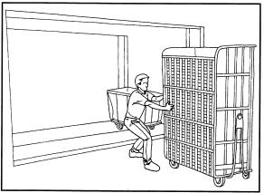
To position loads in and out of the elevator, always stand at the corner, facing your load at a 45° angle with wide stance. Remember to move your close foot to the side of the load to avoid running over it. Next, hang on low on the load. The lower you grasp the load, the lower you are going to be able to place your body when pulling.
