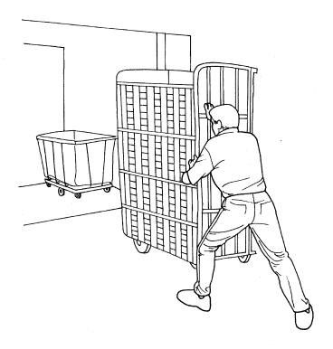
Pushing loads to and from the elevator require the same wide stance POWERLIFT® technique. Here, stand at the back corner of the load, but remember to keep a very wide stance as you push. Once again, keep yourself low to the load instead of way up high as this allows your legs to dig in and take the brunt of the pushing power.
