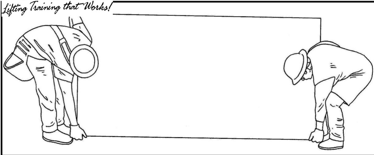
In observing these workers, you can truly see that they both are using a narrow stance and a back lift to transfer this sheet of Gypsum.
