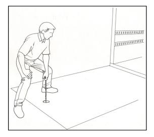
To raise the dock plate, step over the chain with one foot on the dock plate and one foot on the floor. This will allow you to create a wide stance POWERLIFT® position. With your free hand on your leg, lower yourself down and pull the chain with POWERLIFT®.
