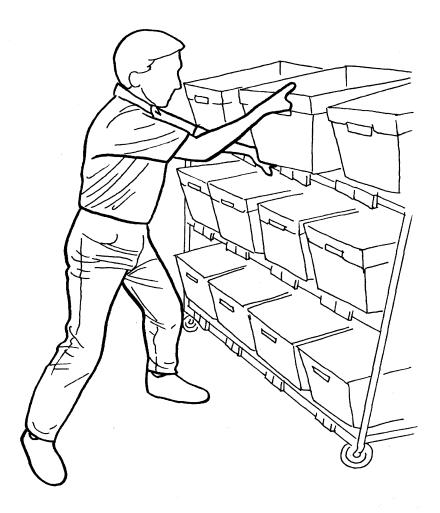
Pulling Tubs and Trays from racks can be made much easier with a few simple techniques. First, instead of lifting the tub or tray from the rack, learn to slide it. Second, if the tub or tray is on a high rack or is heavy, learn to use your free hand to push against the rack as you pull the load towards you with your opposite hand.
