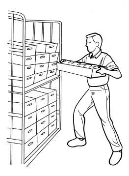
When pulling loads from the top of the APC, try this method. Stand in a wide stance at an angle to the front of the APC and pull the load to you with one hand, while pushing off with the opposite hand. As the tub or tray moves to the edge, catch it's opposite handle with your free hand prior to the tray dropping. Avoid the strain of a sudden impact of the load.
