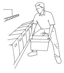
As soon as the empty tub has been positioned, take your right hand from the empty tub and reach down for the handle of the full tub, which is sitting on the floor between your feet. You are now in a perfect position to POWERLIFT® the full tub off the floor and walk away with it.
