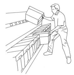
A good way to pull and replace a flat tub at the AFCS is with the following technique. First, as seen in the illustration to the left, stand with a wide stance facing the AFCS at a 45° angle. In this case the empty tub is being held in the right hand, while the left hand pulls the full flat tub from the machine.
