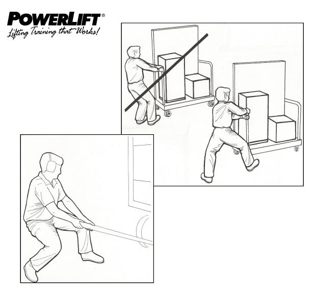
When pulling, use the same stance you would use if you were in a Tug of War contest. Pull from the front of the cart at a 45° angle to the handle utilizing wide stance. Use your legs to pull the cart, not your back. To get the cart moving, pull with a moderate, steady pressure, rather than several sudden jerks. To stop a heavy cart, step in front of the cart with a wide stance, 45° angle to the cart, and use your legs to stop the momentum of the forward moving cart.
